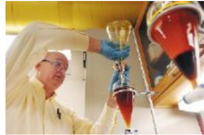
By Nirmalendu Majumdar/The Tribune Matt White, oleo chemical engineer at Renewable Energy Group, separates refined biodiesel and biomass from crude algae oil at the Iowa State Food Sciences Building Tuesday in Ames.
